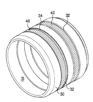
(57) Abstract: Drum device for a home appliance having a chamber (31) for drying or washing laundry, including a sound attenuation member (40) fitted to an outside surface thereof, thereby effectively attenuating noise caused by impact of articles, such as buttons, zippers, clips, and the like fitted to the laundry, to the metallic drum when the laundry introduced into the chamber is lifted and dropped as the drum rotates.
