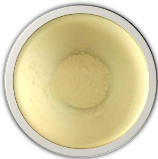
Fig. 2 Fine SnO 2 powder prepared via hydrothermal synthesis.
