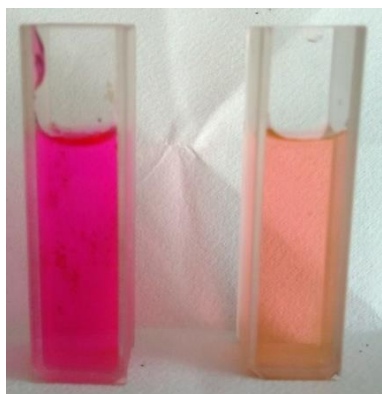
Fig.5 Photograph of RhB before the irradiation and after 2 h.
