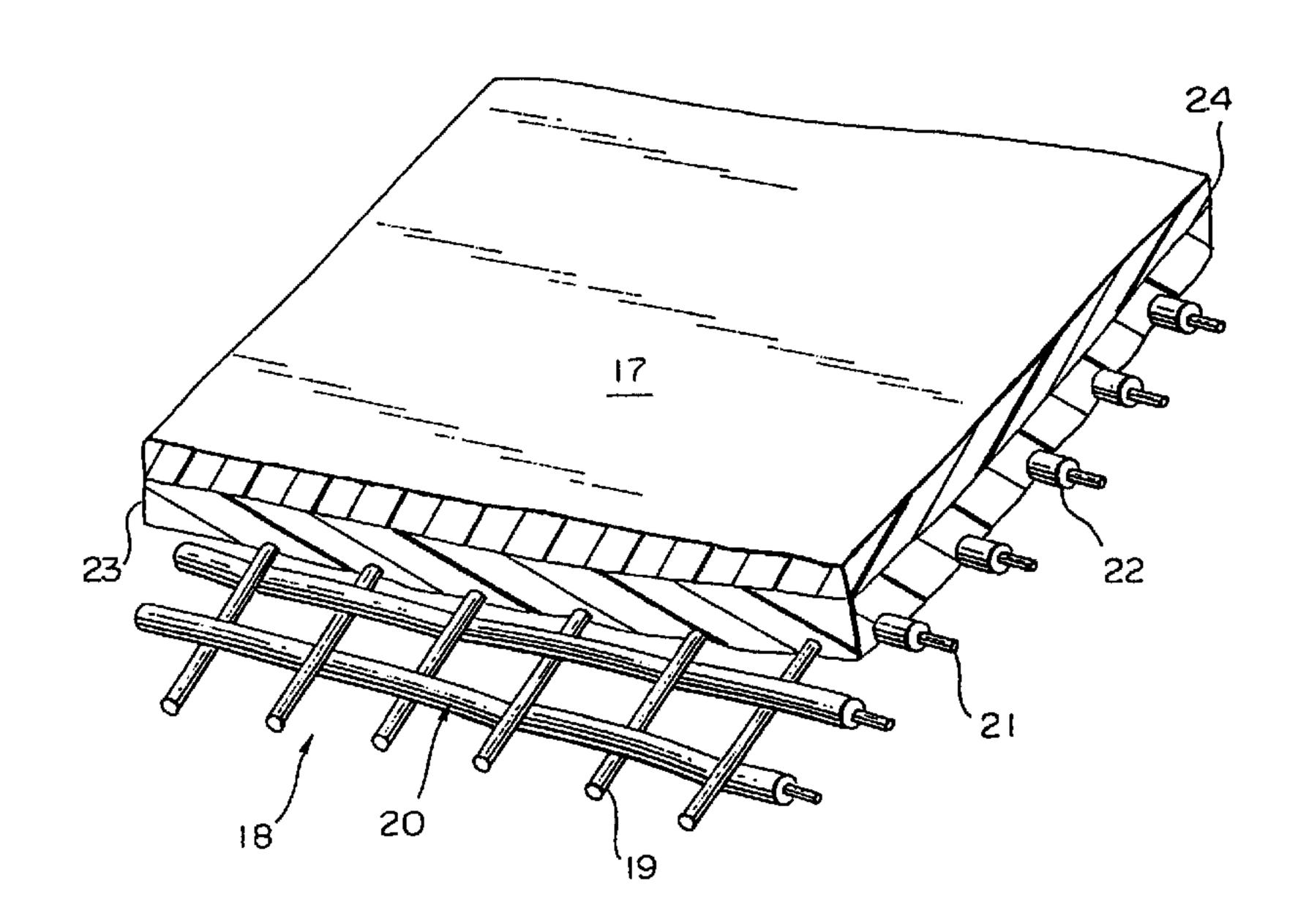
(57) The following describes elasticized artificial leather characterized in that it is formed by a woven support material comprising warp threads and weft threads, said material being coated on at least one of its two sides by at least one layer of synthetic polymer, said woven material having its weft made from elasticized yarn produced using elastomeric fibers. A further object of the present invention is a process for production of the elasticized artificial leather.
