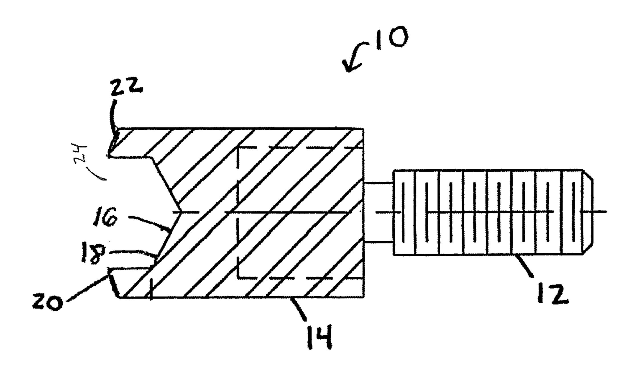
(57) Abstract: The present invention is directed to a welding tip (10) for welding polymeric materials such as containers. The welding tip (10) includes a cylindrical body (14) having a central bore (16) and includes a perimeter (20) around the bore (16).
