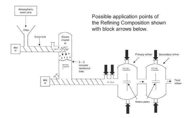
Third refiner Secondary refiner the Refining Composition shown Possible application points of 35% Pulp consistency Primary refiner Refiner plates with block arrows below. \* 30 - 50 psi minutes residence time 2-3 Steam chamb 50% Pulp consistenc y ä Mag or Screw feed Atmospheric wash tank Chips Mot
