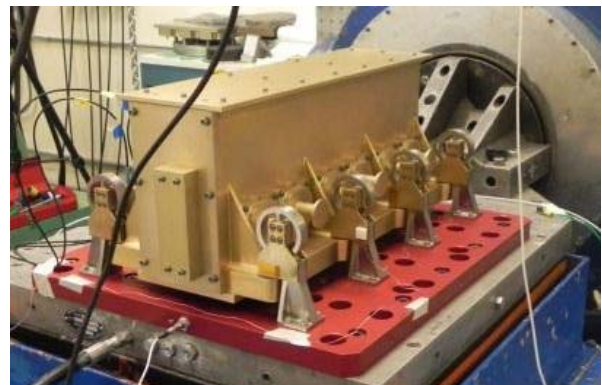
Figure 10. DAA test configuration showing isolator orientation. (photo taken at Moog-CSA Engineering Facility)
