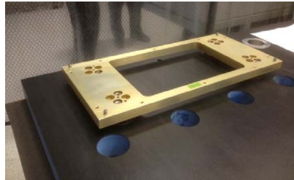
Figure 7. DEM Frame Used to Position Structure Panel Inserts During Bonding Process (photo taken at NASA GSFC)
