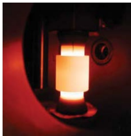
Figure 2: Sintering at high temperature using FAST at Applied Research Laboratory, Pennsylvania State University.
