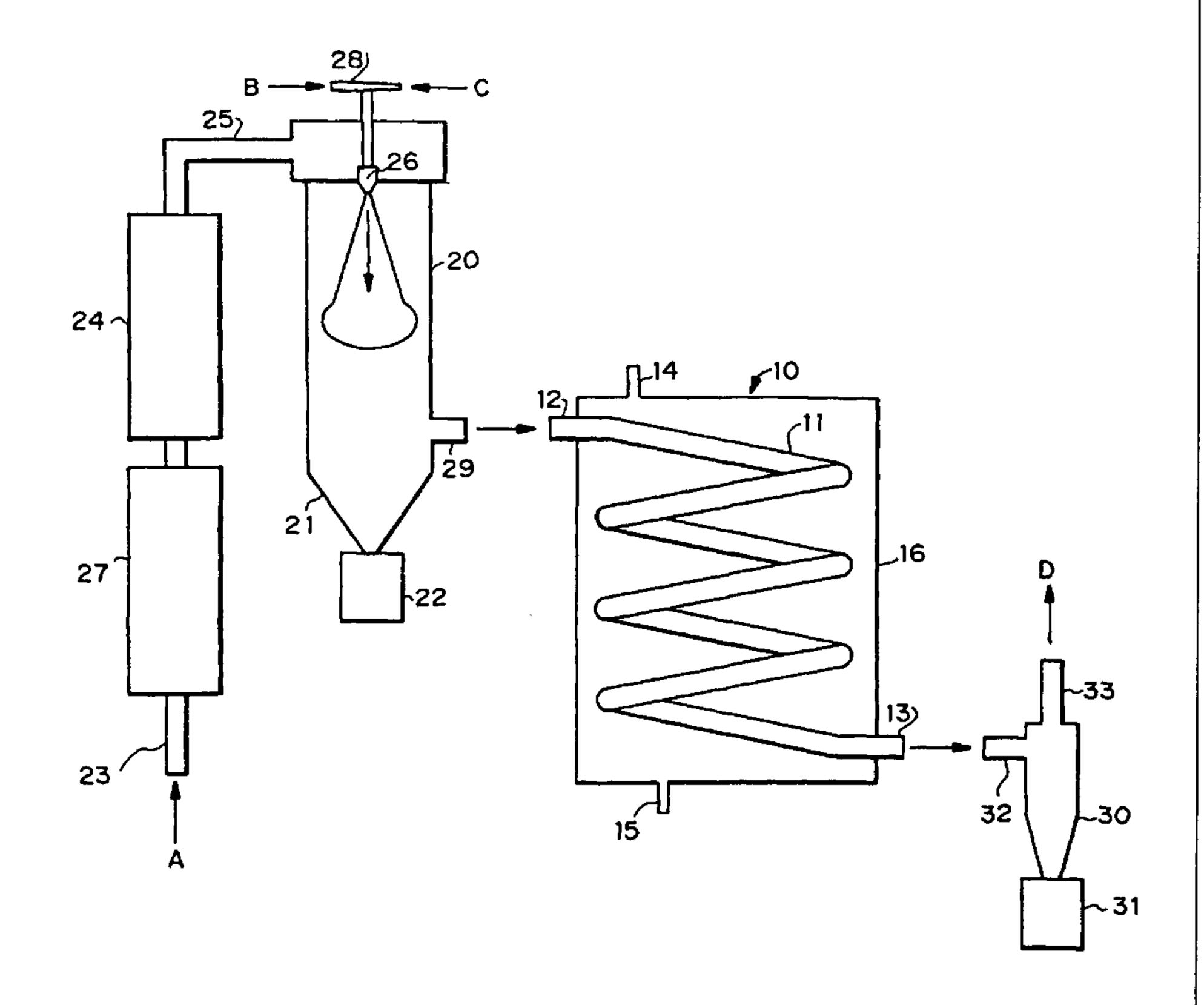
quirements, and may optionally include a jacket to control the temperature of the secondary drying process. A preferred application for the spray drying process and equipment is in the production of microparticles, between about 1 and 200  $\mu$ m in diameter, which can be used to deliver therapeutic and diagnostic agents.
