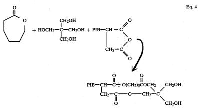
when a  $C_5-C_9$  lactone, such as E-caprolactone is heated simultaneously with a polyamine, such as 1,2-diaminoe- 50 thane, and with an acrylating agent, such as polyisobutenyl succinic anhydride, the reaction mass will comprise a mixture of dispersants which contain a sequence of methylene units which is derived from the lactone reagents. In the case of E-caprolactone, which is a pre- 55 of dispersant products is illustrated.) ferred lactone for use in this invention, the dispersant
