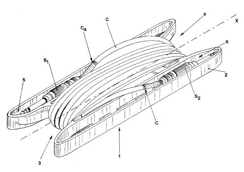
(57) Abstract: A winding device (1; 100) for the connecting cables (C) of electric and/or electronic equipment and/or instruments comprising a frame (2; 101) which mainly extends according to a longitudinal axis of symmetry (X) and in which there is a pair of first housings (3, 4; 120, 121) positioned opposite one another, which hold the cable (C), and second housings (5, 6; 118, 119) which hold the jacks (S1, S2) connected to the ends (Ca, Cb) of the cable (C).
