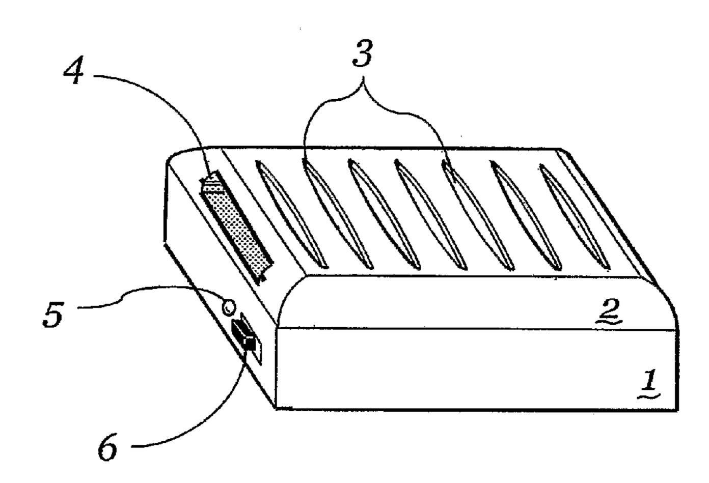
(57) Abstract: A device for enabling vapourization of a chemical formulation into an atmosphere comprising means (4) for receiving a cartridge including the chemical formulation, aperture means (3) to enable vapourized chemical formulation to be guided therethrough into the atmosphere, wherein the chemical formulation contacts a heater means in order to vapourize the chemical formulation.
