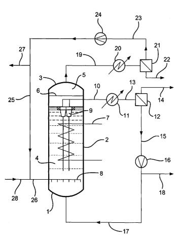
(57) Abstract: A process for the production of liquid hydrocarbon products by passing, at elevated temperature and pressure, synthesis gas and a fluidising liquid through a fluidised catalytic bed within a reaction zone, characterised in that the fluidised catalytic bed is an aggregative fluidised catalytic bed comprising a particulate Fischer-Tropsch catalyst having a density of greater than 4,000 kg/m<sup>3</sup>.
