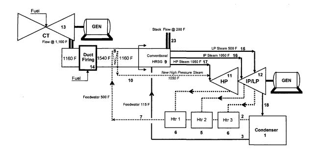
Method To Integrate Regenerative Rankine Cycle Into Combined Cycle Applications
