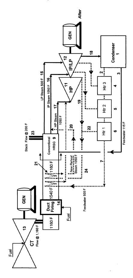
Method To Integrate Regenerative Rankine Cycle Into Combined Cycle Applications **Drawing 3**
