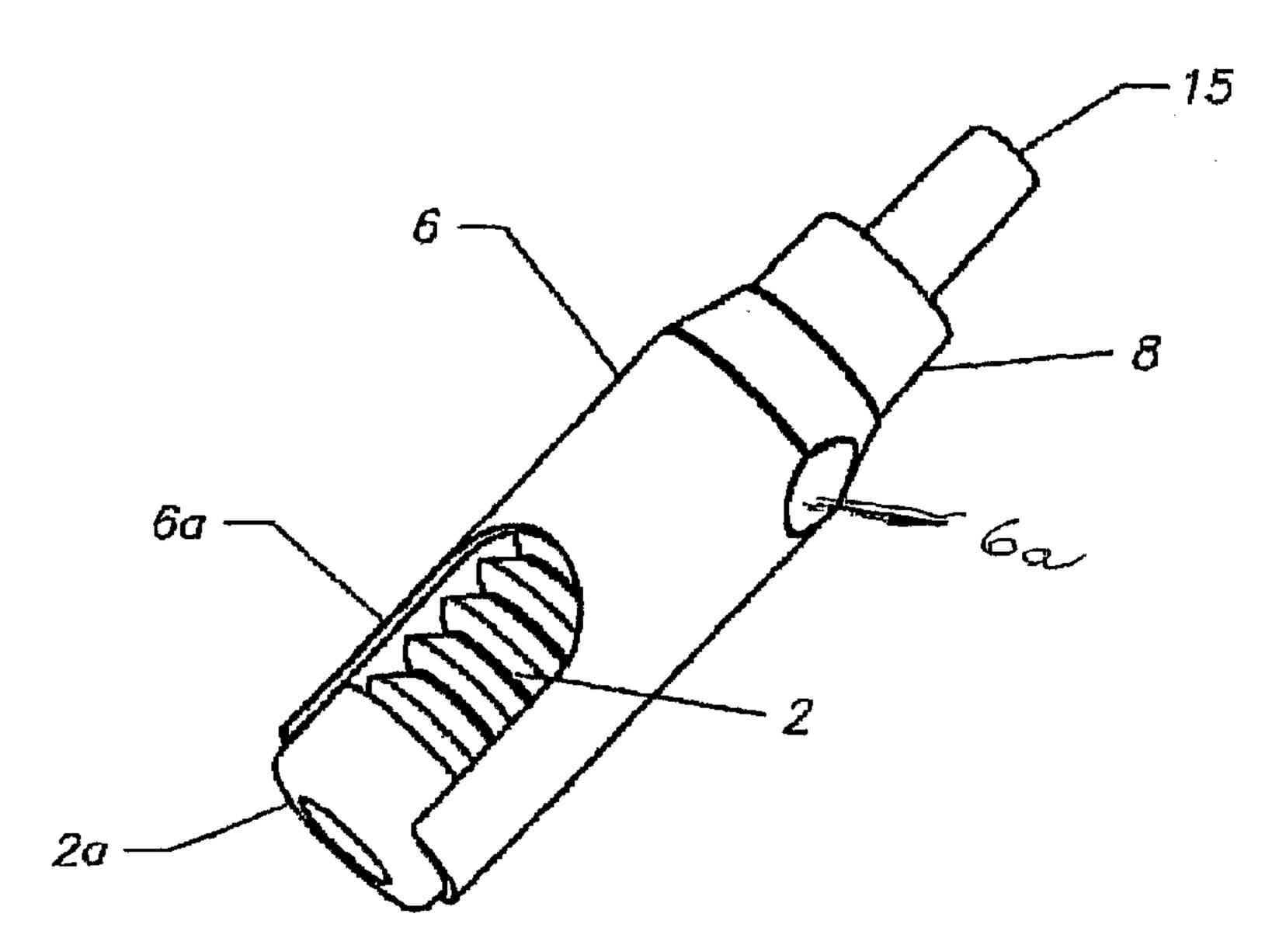
(57) Abstract: A one way valve assembly flows a sterile flowable substance from a source to an outlet orifice and prevents any backflow of contaminants through the one way valve assembly when the flowable substance ceases to flow. The valve assembly includes an elastomeric membrane which aids in preventing any backflow of contaminants when dispensing of the flowable substance is stopped.
