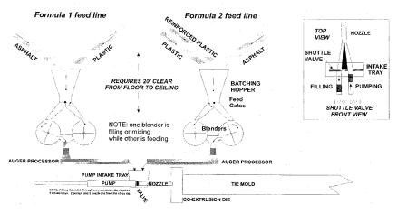
(57) Abstract: Durable, weather and insect resistant railway tie fabricated from at least one composite extrudable composition comprising an asphaltic portion and a polymeric portion comprising a mixture of recyclable plastics and a strengthening filler agent such as glass fibre or Kevlar®. The said composite railway tie is manufactured by moulding the railway tie core using a first extrudable composition and moulding the outer portion of the railway tie using a second extrudable composition.
