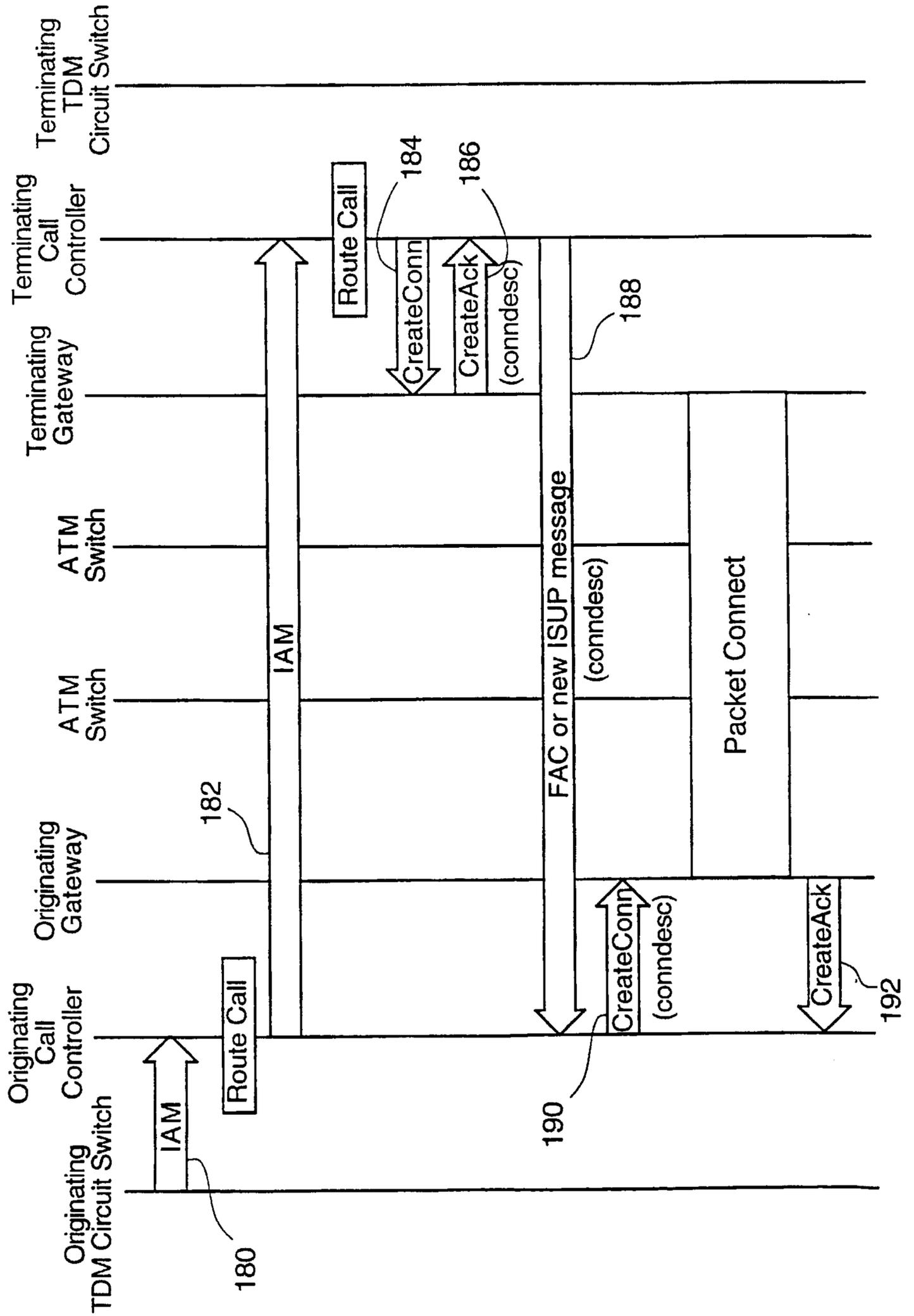
FIG. 8 Call Scenario for Multiple Calls associated with one VCC:
