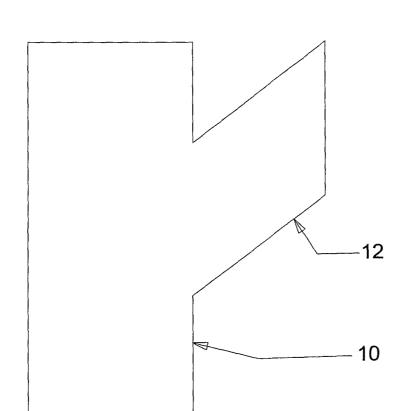
(57) Abstract: A plumbing unit includes a length of flush pipe (10) and a vent pipe comprising a length of a standard diameter pipe (12) joined to the flush pipe at an angle in the form of a Y-piece.
