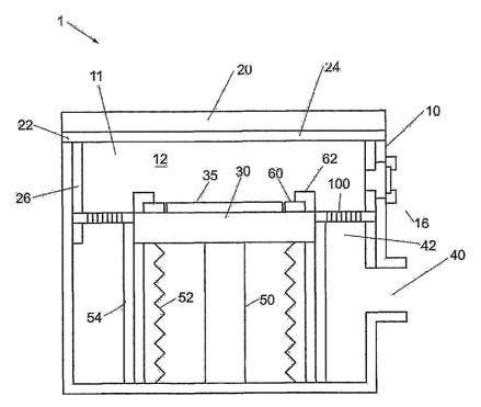
(57) Abstract: The present invention presents a baffle assembly located in a plasma processing system, comprising a baffle carrier attached to the plasma processing system, and at least two baffle inserts having a plurality of passages therethrough, the at least two baffle inserts being supported by the baffle carrier.
