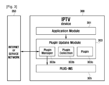
(57) Abstract: A method and system for updating a plug-in in a device in Internet Protocol TeleVision (IPTV) system are provided. The method includes determining a second plug-in group selected from among a first plug-in group to be updated according to status information of each plug-in indicated in the first plug-in group in the device; and updating each plug-indicated in the determined second plug-in group.
