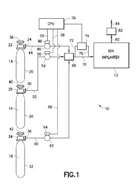
(57) Abstract: Ion implantation compositions, systems and methods are described, for implantation of dopant species. Specific selenium dopant source compositions are described, as well as the use of coflow gases to achieve advantages in implant system characteristics such as recipe transition, beam stability, source life, beam uniformity, beam current, and cost of ownership.
