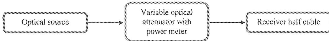
Fig. 1: Schematic for test to measure receiver coupling efficiency of a half cable
