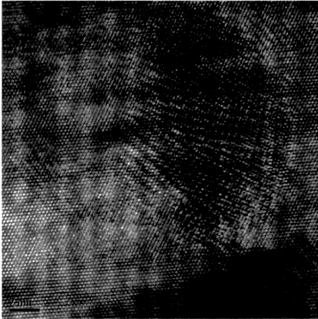
High-resolution morphology and size of Cu precipitates
