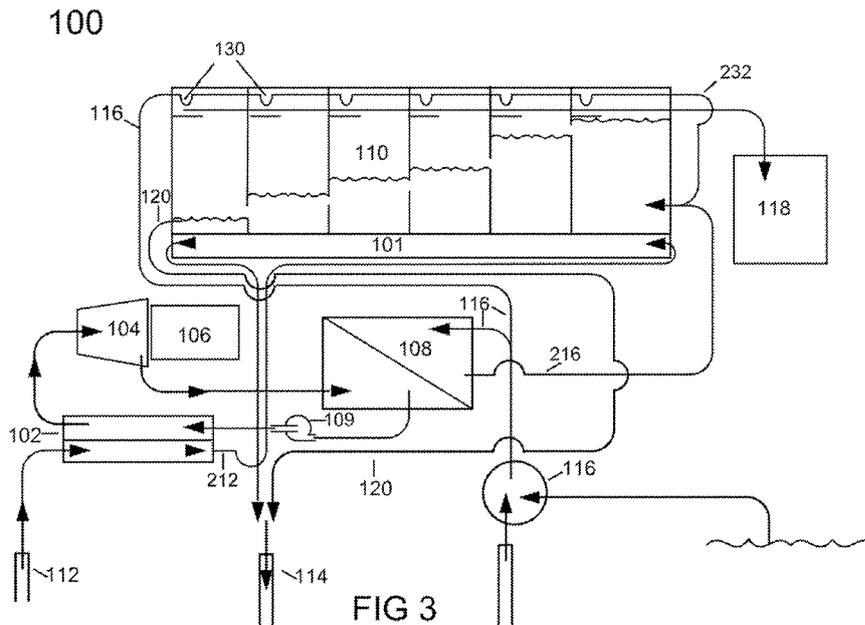
(57) Abstract: A method and apparatus for implementing the Rankine Cycle with improved efficiency through the use of thermal exchange between the working fluid and a brine liquid. In one embodiment, the brine liquid is further processed through a multistage flash distillation unit to produce distilled water or other minerals. Geothermal or exhaust waste heat may be used to further improve the Rankine Cycle efficiency, with remaining thermal energy improving the distillation process.
