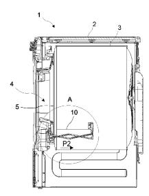
(57) **Abstract:** The present invention relates to a laundry dryer (1) comprising a body (2); a drum (3) which is placed into the body (2) and wherein the laundry is loaded; a loading opening (4) which is provided on the body (2) and which provides access into the drum (3); and a front bearing (5) which rotatably supports the drum (3) and whereon the loading opening (4) is provided.
