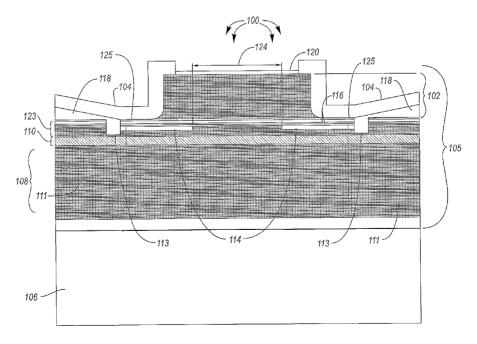
(57) Abstract: An electro-absorption modulator integrated with a vertical cavity surface emitting laser (VCSEL). An electro-absorption modulator (EAM) is integrated or grown on a VCSEL. The electro-absorption modulator may be separated from the VCSEL by a semi- insulating or nonconducting layer. Contacts on the EAM can bias the EAM such that 0 light emitted by the VCSEL is selectively absorbed. Thus, the VCSEL can emit a constant wave light that is modulated by the integrated EAM.
