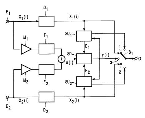
(57) Abstract: A method and arrangement for bit-synchronizing a  $\Sigma\Delta$ -modulator with pre-filter to an incoming single bit bitstream. One or more of the integrator states of the  $\Sigma\Delta$ -modulator are corrected by a signal which is calculated from the incoming bitstream and at least one of the pre-filtered input signal and the output bitstream of the  $\Sigma\Delta$ -modulator.
