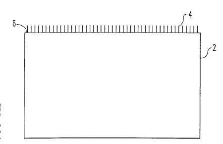
(57) Abstract: This invention discloses a bag or wrap having hair like protrusions (4) extending substantially perpendicular to a surface (6) of the bag or wrap thereby enabling the bag or wrap to attach or cling to other surfaces. This invention also discloses a method of making a bag or wrap having the hair like protrusions (4).
