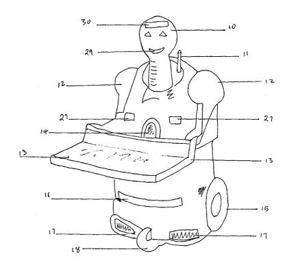
housing (fig. 1. 10) and will be run on collective energy as well as electricall powered no wires will be resticting the Robo-nurse for the safest of operation. The Robo-nurse can be activated by the pager receiver (fig. 1. 11) by remote control or by voice activating commands. The body and shoulders wil be padded (fig. 1. 12) to give comfort to the patient, the tyres will be of non slip rubber (fig. 1. 15).
