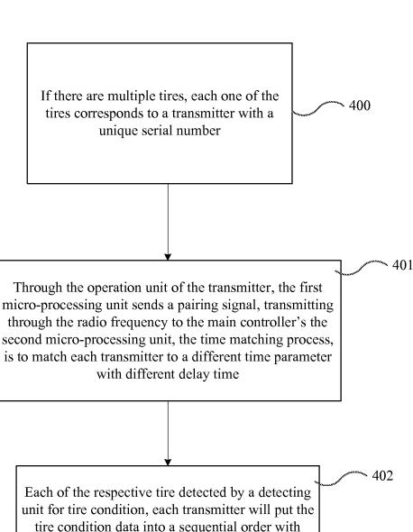
Each of the respective tire detected by a detecting unit for tire condition, each transmitter will put the tire condition data into a sequential order with different delay time, through the radio transmission, this information is transmitted to the main controller of the second micro-processing unit
