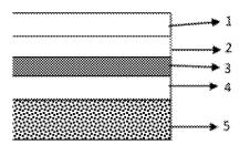
In the figure: layer 1 is the adhesive layer Layer 2 is the barrier layer Layer 3 is the base layer Layer 4 is the barrier layer Layer 5 is the high-reflection layer
