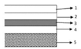
In the figure: layer 1 is the adhesive layer Layer 2 is the barrier layer Layer 3 is the base layer
