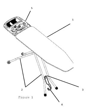
(57) **Abstract:** The invention is related with an ironing board which has a hanger apparatus (4) associated with the legs (2) of the ironing board that are connected to the ironing surface (1) in order to enable opening and closing of the ironing board.
