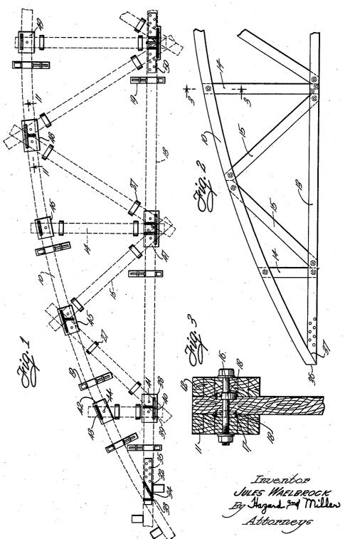
TEMPLATE FOR FASHIONING ELEMENTS OF ROOF TRUSSES AND LIKE STRUCTURES
