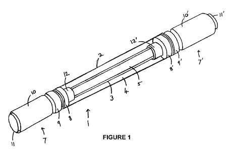
(57) Abstract: A directional gas pressure device (1) comprises a body (2) having openings at each end thereof, a closure member (7) for each end thereof, a tie member extending through the body, the closure members (5) being attached to the tie member. The closure members are adapted to increase their size upon evolution of gas from a pyrotechnic charge material contained within the body.
