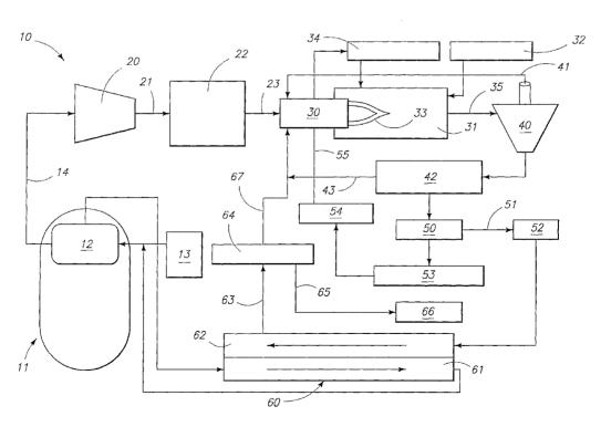
(57) Abstract: A method for forming ammonia is disclosed and which includes the steps of forming a plasma; providing a source of metal particles, and supplying the metal particles to the plasma to form metal nitride particles; and providing a substance, and reacting the metal nitride particles with the substance to produce ammonia, and an oxide byproduct.
