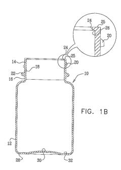
(57) Abstract: A plastic container including an outer container element (10) having a geometrical center and an inner container element (50) mounted within the outer container element, the outer container element and the inner container element, when mounted in the outer container element, together having a center of gravity which is lower than the said geometrical center of the outer container element.
