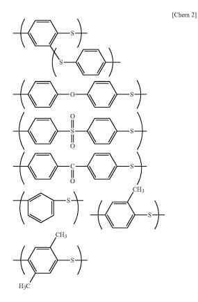
**[0026]** Since the PPS copolymer (A) having such a structure partially has a low melting point, the resulting resin composition is advantageous in formability.
