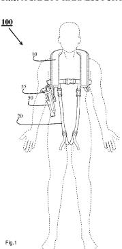
(57) **Abstract:** A safety apparatus for rock fishing comprising: a life-jacket including a harness, the harness having three fixing points; a tether for restraining a user, in use, and an anchor for securing the tether to land.
