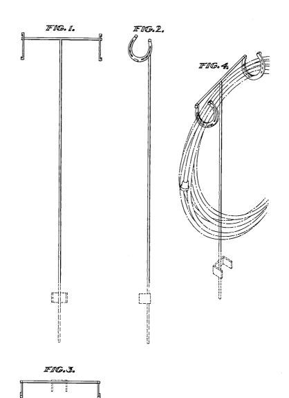
FIG. 1 is a front elevational view of a hose coil holder embodying my new design.
