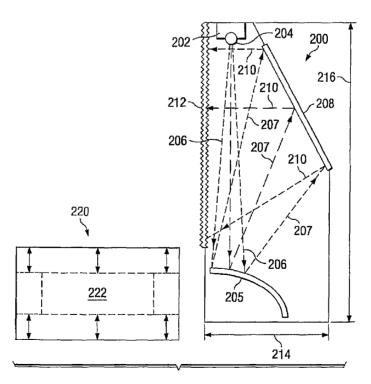
(57) Abstract: Described is a rear projection television (200) with reduced cabinet depth (214) and method of manufacturing thereof. An anamorphic projection lens (204) compresses an image and projects it along an optic path, where a cylindrical mirror expands and reflects the image within the optic path. The combination of compression and expansion facilitates in the design of a rear projection television with reduced cabinet depth.
