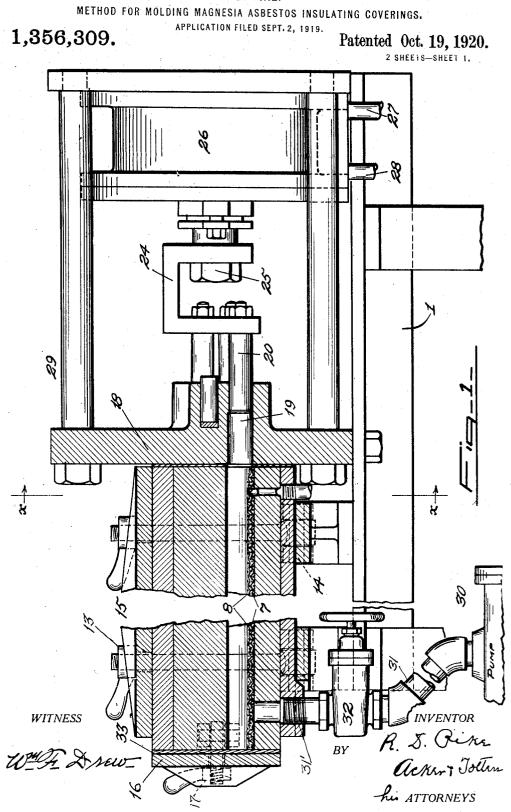
R. D. PIKE. METHOD FOR MOLDING MAGNESIA ASBESTOS INSULATING COVERINGS.
