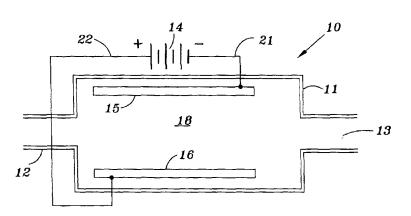
(57) Abstract: The shelf life of a comestible liquid is prolonged by passing the liquid through an electrolytic cell. Electric current travels from one electrode to the other through the liquid. The electric current destroys bacteria present in the liquid. The current causes the osmotic balance of the bacteria cells to be disrupted causing the cell to either implode or explode.
