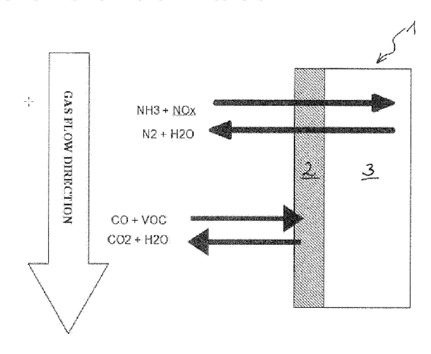
(57) Abstract: A method and a catalyst, where flue gas or exhaust gas containing harmful carbon monoxide, organic compounds (VOC) and NOx is contacted with a layered catalyst in which a first layer comprises an oxidation catalyst and in an underlying layer a NH3-SCR catalyst for the simultaneous removal of the carbon monoxide and NOx.
