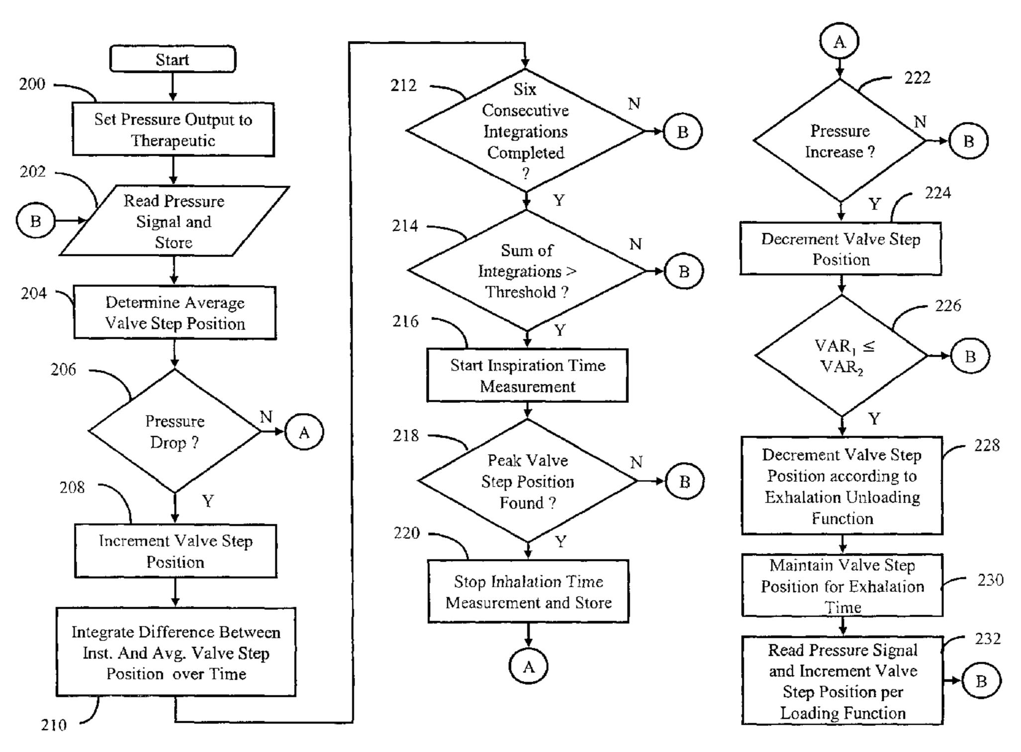
(57) Abstract: Systems and methods of providing a breathing gas are provided. The method includes, for example, sensing a parameter associated with the delivery of a breathing gas, changing a valve position in response to a change in the sensed parameter, determining a breathing state based on the valve position, and causing a change in the sensed parameter of the breathing gas based on the determined breathing state.
